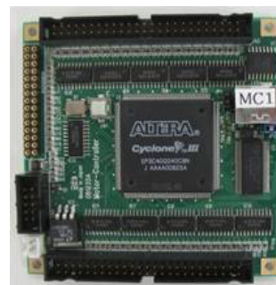
Motor Controller (FPGA Cyclone III)
