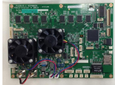
Image Processing Board (ARM TI8168 Cortex-A8)
